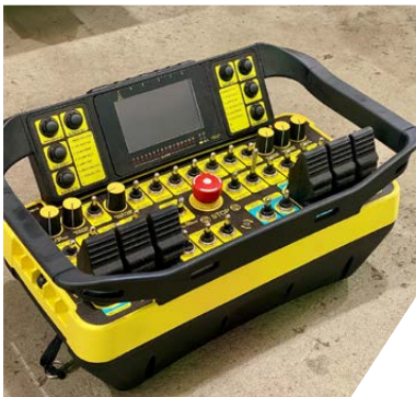
Wireless Remote Control Transmitter (WRCT) for Rig 29 – NGBF 800 55T pullback Hydro Rig.
