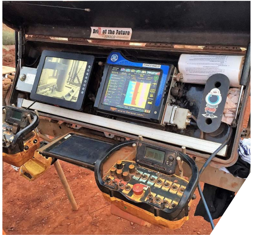
Rig camera screen on LH side and MWD screen on RH side.
